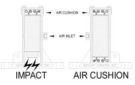
Impacting units provide the most force, but also produce higher noise levels. Air Cushioned (nonimpacting) models feature lower noise levels, but produce less force. When replacing an Impacting unit with an Air Cushioned, it may be necessary to use a larger model, or additional vibrators to achieve proper material flow. Consult HV for assistance in selecting the proper model to suit your location.
