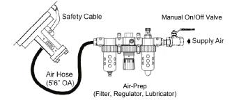
Single-unit manual installation for bins and hoppers is shown here for reference purposes.
